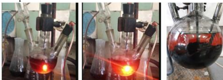
Fig. 1. Synthesis of spherical carbon nanoparticles by the high-frequency discharge-pulse method.
